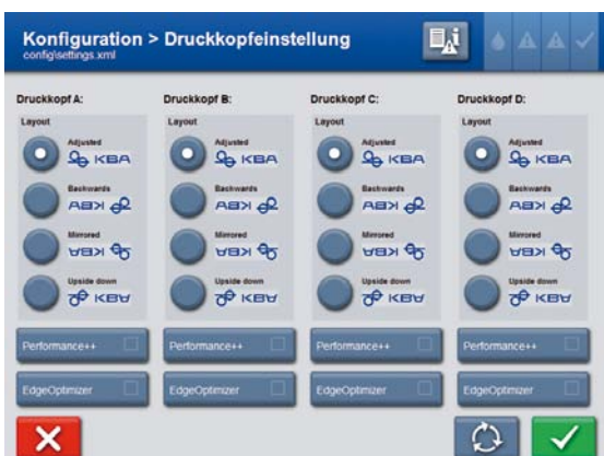
Printing parameters are individual adjustable for each print head
